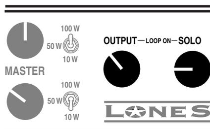
Should you ever use your **LONE STAR** amplifier as a power amp alone by inserting a signal into the RETURN jack, the **OUTPUT** control will serve as the master level control.
