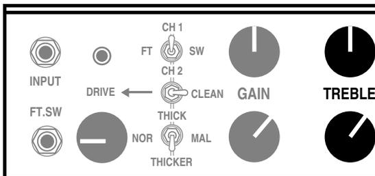
Like most of the controls on your **LONE STAR**, there is an optimum region of the **TREBLE** control where ample top end is mixed in and yet enough signal is still passed on to the **MIDDLE** and **BASS** controls.
