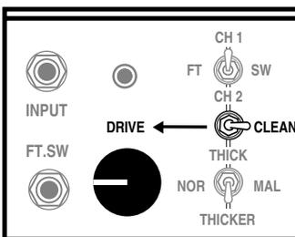
Set to **CLEAN**, all overdrive circuitry is removed and Channel 2 is a slightly higher gain clone of Channel 1. Because of this additional gain in what is otherwise a “rhythm” circuit, Channel 2 is an amazing solo channel for Roots style rhythm work or howling blues solo sounds. Cranking the GAIN control in Channel 2 **CLEAN** is a wonderful alternative to the more saturated sound of the **DRIVE** circuit.
