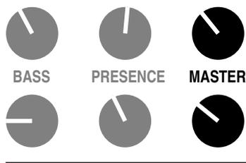
Again, we suggest using the **MASTER** control in its *sensible* ranges ( 9:00 - 2:00 ). Here, the channels will be easier to match with each other and the Effects Loop will see more reasonable signal levels.
