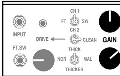
In most guitar amplifiers, and especially in all-tube circuits, the **GAIN** control is the most powerful control in the preamp. It shapes the overall style and character of the sound and is responsible for whether the sound is clean, overdriven or anywhere in between. In your **LONE STAR** the **GAIN** control is even more powerful. It not only determines the amount of drive, but also acts as an integral part of the tone control string as well.
