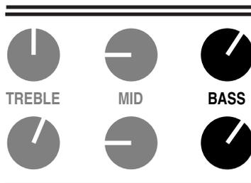
For the most balanced sound and a balance of power between the three rotary tone controls, try to use the **TREBLE** control in its middle ranges. This scenario produces nearly equal representation of all the frequencies on the tone controls and provides a great neutral starting point for further tweaking.
