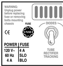
If you see nothing abnormal when you switch the STANDBY on, it is possible that a power tube shorted temporarily and blew the **FUSE**. If this is the case it may work again normally. To be safe, you might want to replace just the adjacent tube or all power tubes in the "shotgun" troubleshooting tradition and save the replaced set as spares. Spare fuses are a must for the fabled cord bag along with your spare tubes. Always carry both for they could be worth their weight in gold someday.
