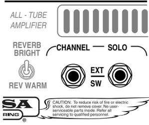
The **EXTERNAL SWITCH** jacks respond to any tip-to-ground latching type logic for their triggering. This type of switching logic can be found on most midi master control switching units on the market.
